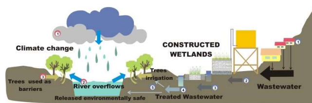
Figure 1: Treatment of sewage and high Andean plants acting as natural barriers.
